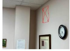
One satellite would be mounted high up on the wall in the MMB large classroom at the end of the hallway near an existing hard-wired LAN jack and power outlet. This location would provide good coverage for the back rooms in the MMB.
