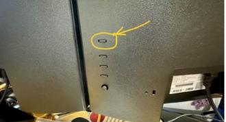
The monitor ON/OFF switch is on the BACK of the monitor. It is the small button at the TOP of the stack of buttons.
