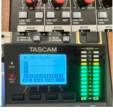
11. Repeat steps 9 & 10 for each channel being recorded noting that you may have to switch the LCD display screen to channels 9-16 to see channels above channels 1-8. Use the second and third black buttons immediately beneath the LCD display screen to select the channels you want to see.
