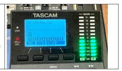
9. Using the red GAIN knob at the top of each channel strip, adjust the gain on each channel to get a meter response in the -20dB to 0 dB range.
