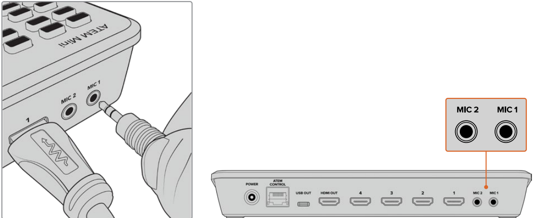
Connect microphones to ATEM Mini's mic inputs
